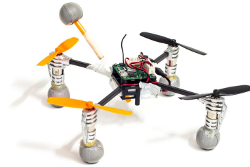
Figure 1: Modified Walkera Ladybird with markers for the tracking system.
